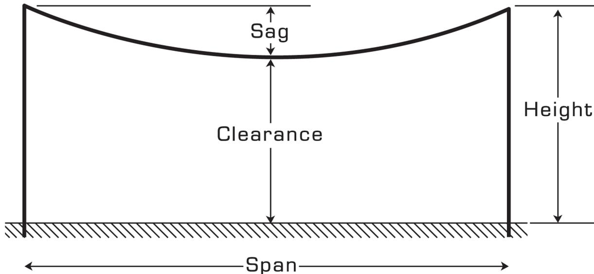
Preliminary design is usually a matter of assigning values to the dimensions shown in Figure A.
